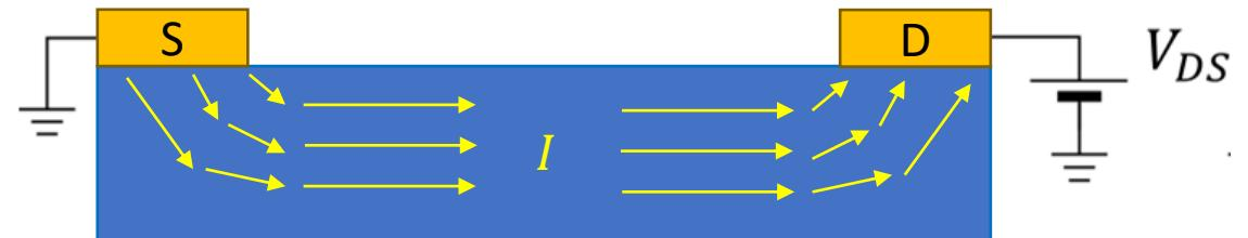
$$\text{In general: } R_{TOT} = R_{sc} + 2R_c + 2R_m$$
